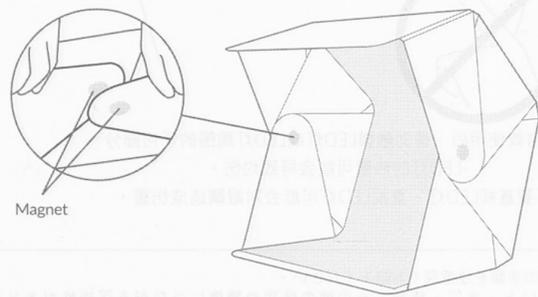
② Install the backdrop inside the Foldio3. Take note that the backdrop installation is different depending on the color of the backdrop.
